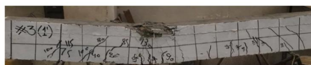
Crack pattern of group (2B)
