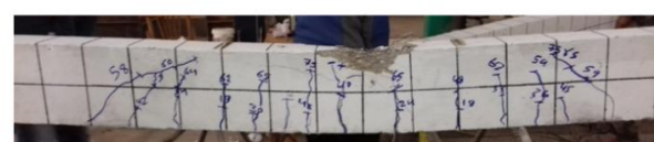
Crack pattern of group (1A)
