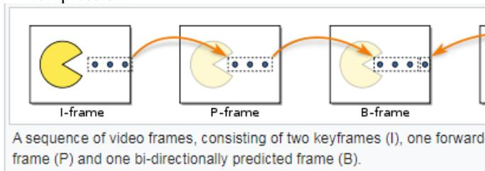
Three types of pictures (or frames) are used in video compression: I, P, and B frames.
