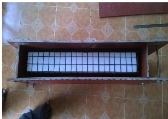
**Weld mesh thermocol with r/f**
