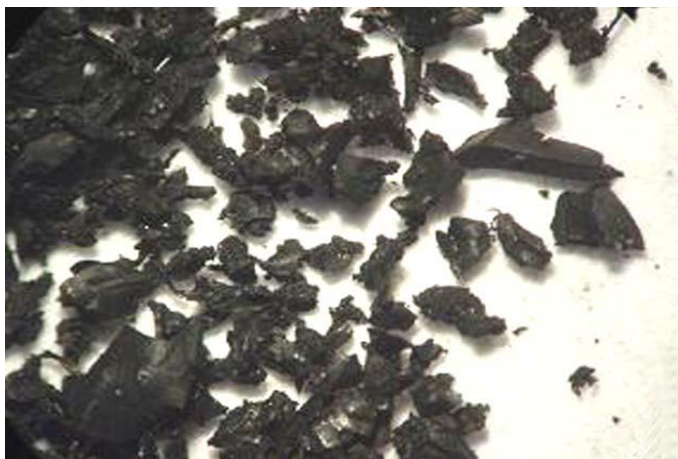
Figure 3: The Rubber particles by a stereoscope [32].
