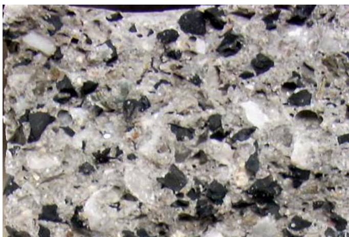
Figure 4: The Rubber distribution in concrete mixture [32].
