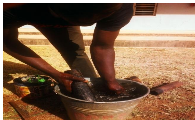
Figure 3: Washing the mild steel pipe
