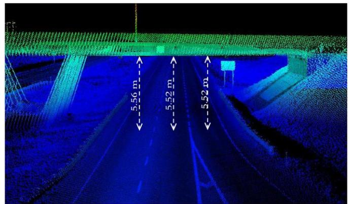
Fig 4: Clearance Using Mobile LiDAR
