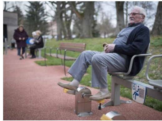
Fig. 4 Cycling ergometer for elderly people operation in outdoors open condition.
