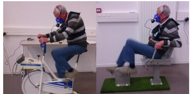
Fig. 1 Oxygen uptake measurements during tests with reference (left) and designed (right) cycle ergometer.
