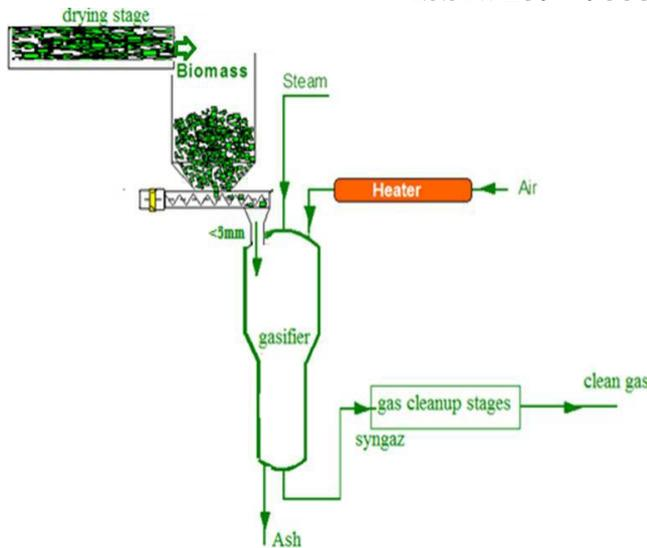
Fig.1 Schema of trained flow gasifier [6]
