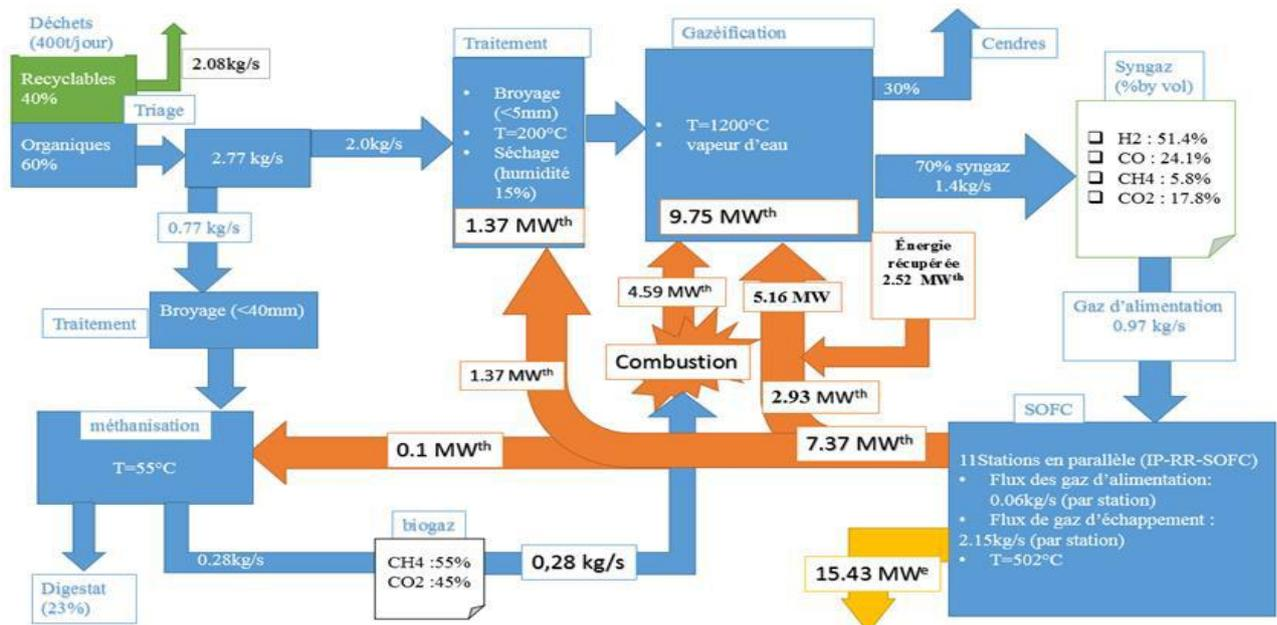
Fig.3 Diagram of the new hybrid solid waste treatment, from sorting to electricity generation
