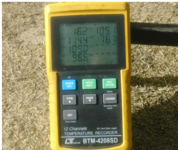
Fig.4. K-Type data logger.
