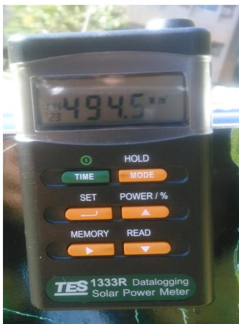
Figure5. Portable solar meter
