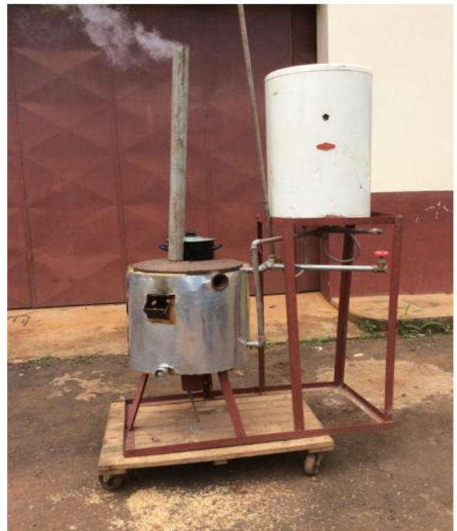
Fig 3 Complete assembled rice husk fired stove
