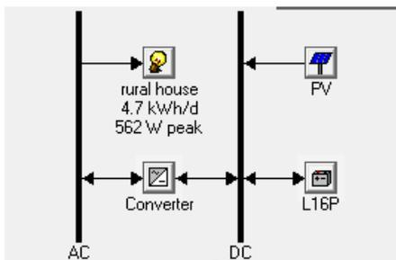
Figure 3: Homer Schematic Diagrams for the PV System
