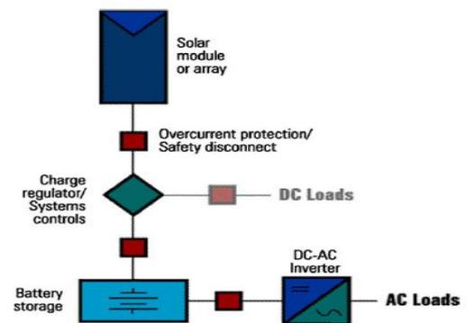
Figure 2: Standalone Photovoltaic System
