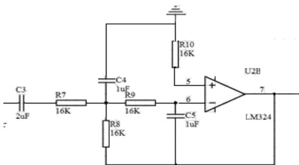
Figure 3: Diagram of the 2nd order low-pass filter circuit.
