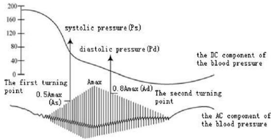
Figure 1: Diagram of the Oscillometric method.
