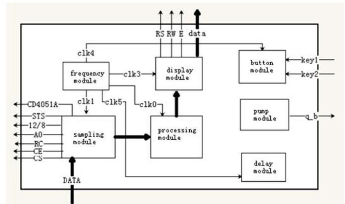
Figure 2: Diagram of the top-level modules in FPGA design
