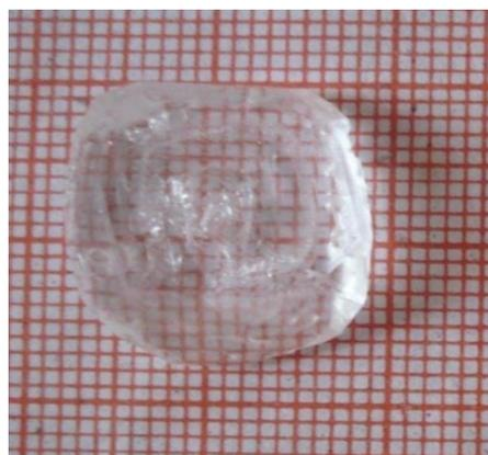
Figure 2: The Photograph of TGS crystal admixture with salicylic acid
