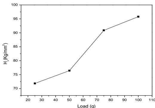
Figure 9: Dependence of hardness number ( $H_v$ ) with load in grams for TGSS crystal.
