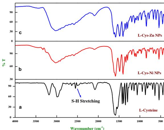
Figure 3: FT-IR spectra of L-Cysteine, L-Cys capped Ni and Zn nanoparticles
