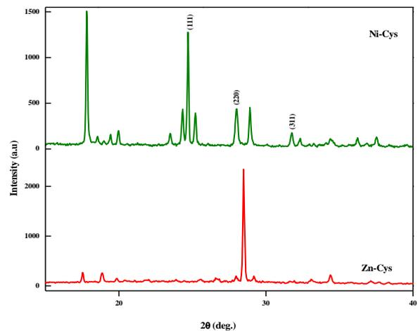
Figure 4: XRD spectrum of L-Cys capped Ni/Zn nanoparticles
