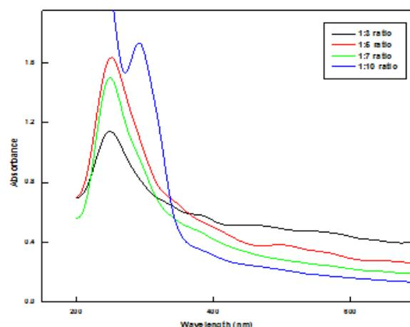
Figure 1: Absorption spectra of synthesized Ni nanoparticles at (1:3, 1:5, 1:7 and 1:10) molar ratios.
