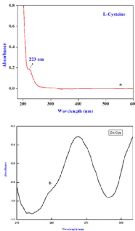
Figure 2: UV-Vis spectra of a) L-Cysteine hydrochloride b) Zn-Cys NPs
