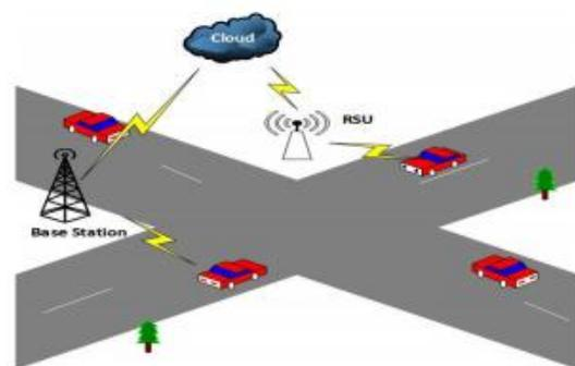
Figure 1: Cloud based architecture
