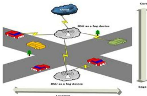
Figure 3: Fog based architecture
