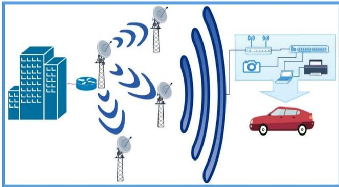
Fig. 6. A Point to Multipoint Access Point Connectivity
