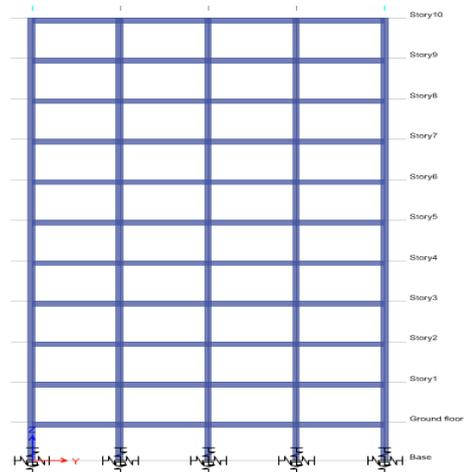
Fig 2.6: Elevation of Bare Frame Model with Flexible Base
