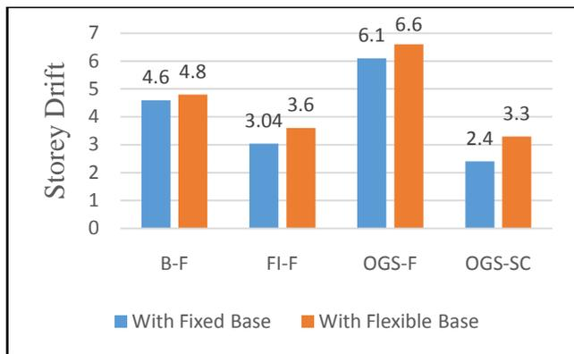
Fig.3.3: Maximum Storey Drift for different Structural forms
