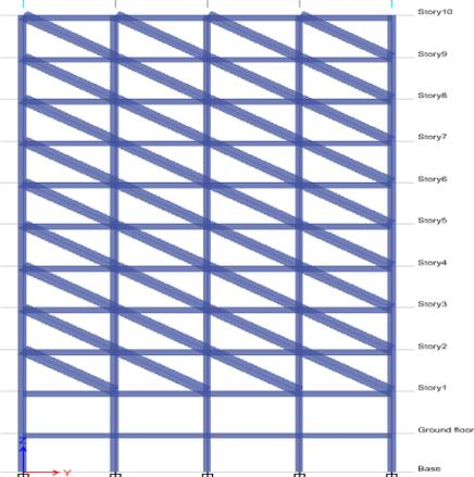
Fig.2.4: Elevation of (OGS-F)
