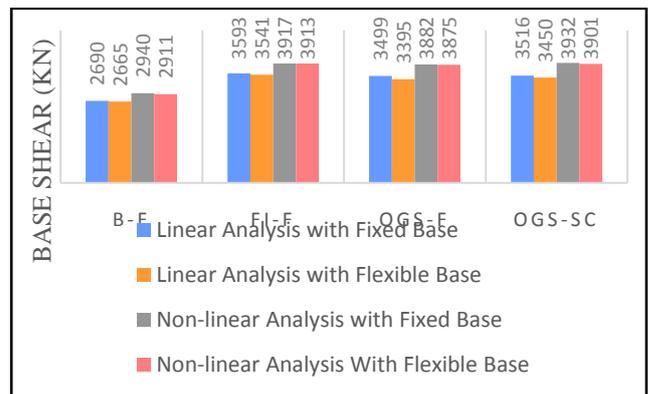
Fig. 3.1: Base shear for different structural forms and analysis.
