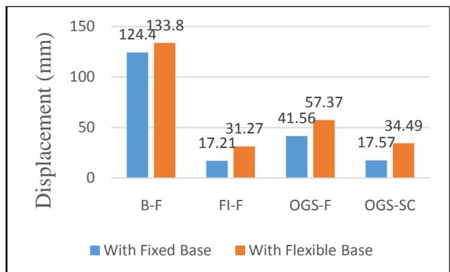
Fig.3.2: Top storey Displacement for different Structural forms
