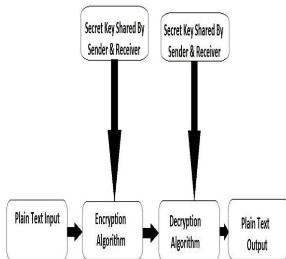
Figure 1: Conventional Encryption Model
