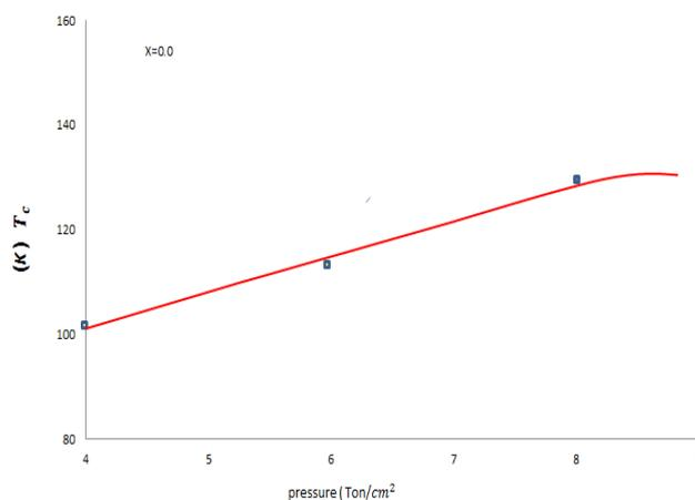
Fig. (2) : critical temperature ( $T_c$ ) as a function of pressure .
