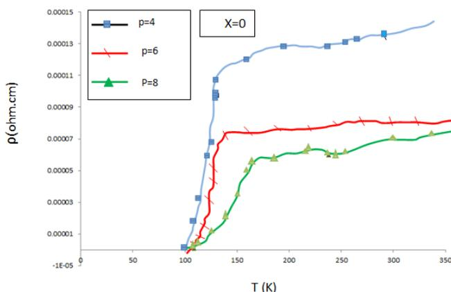
Fig. (1) :temperature dependence of resistivity for  $\text{Hg Ba}_2\text{Ca}_{2-x}\text{La}_x\text{Cu}_3\text{O}_{10+\delta}$  for various pressure in air .
