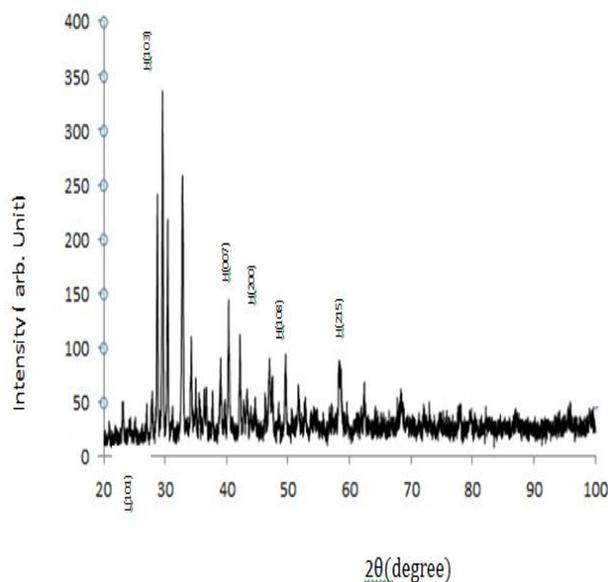
Figure ( 6 ) (XRD) pattern of  $Hg Ba_2Ca_{2-x}La_x Cu_3O_{10+\delta}$  samples For  $x=0.2$  and  $p = 6$
