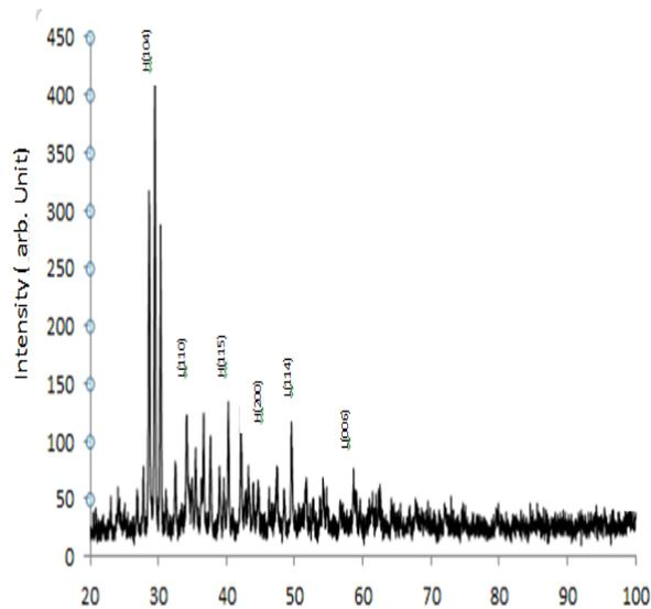
Figure ( 4 ) (XRD) pattern of  $Hg Ba_2Ca_{2-x}La_x Cu_3O_{10+\delta}$  samples For  $x=0$  and  $p = 6 \text{ ton/cm}^2$
