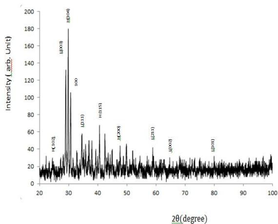
Figure 3: (XRD) pattern of Hg Ba<sub>2</sub>Ca<sub>2-x</sub>La<sub>x</sub> Cu<sub>3</sub>O<sub>10+δ</sub> samples For x=0 and p = 4 ton/cm<sup>2</sup>
